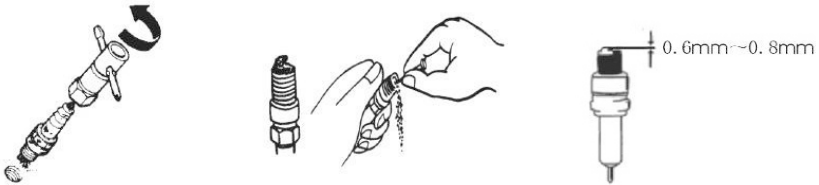
(1) Remove ignition plug (2) Clear off carbon deposit (3) Adjust clearance.
